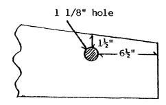
View: R H rear engine baffle, looking forward
